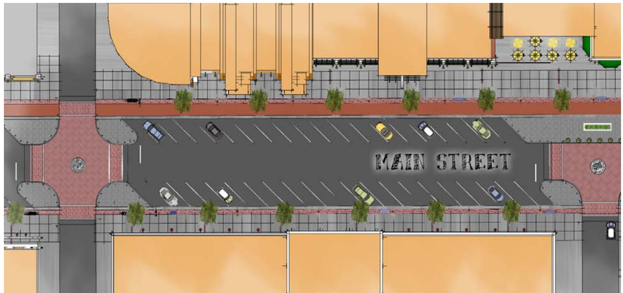
Plan view of Main Street streetscaping project in Speedway, IN which included, pedestrian, bicycle and automobile facilities including raised intersections to slow traffic. (American Structurepoint)
