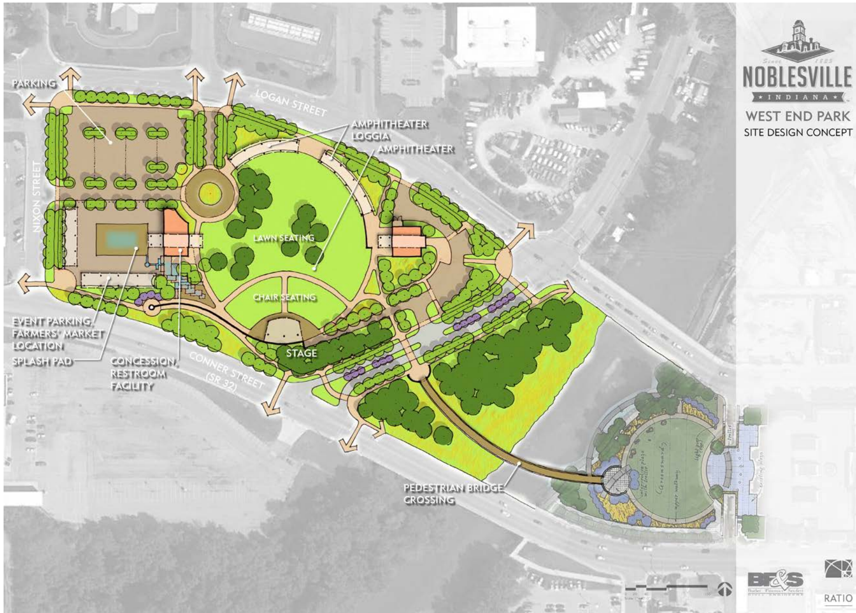
The conceptual West End Park site design includes a new pedestrian bridge to better connect downtown and riverfront recreation areas in the West Gateway.
